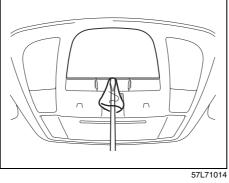
Pull down the lens by using a flat blade screwdriver covered with a soft cloth as shown. To install it, simply push it back in.
